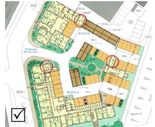
The bin stores serving this East Grinstead block of flats are discretely integrated within the envelope of the building and around the rear courtyard where they avoid deadening the street frontage. They are also well positioned for ease of collection while providing sufficient separation from the adjacent flats to avoid causing undue nuisance
