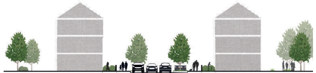
Figure 40: A good formal arrangement for a primary street that incorporates parallel parking with regular tree planting within kerb build outs reducing its impact on the street space (Section)
