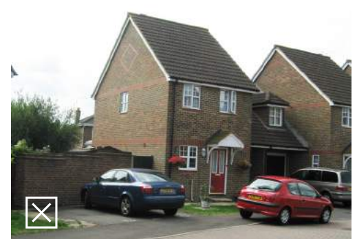
Poorly proportioned detached houses with narrow fronts, deep plans and pitched roofs with high ridge lines generating over-large and mostly blank flanks
