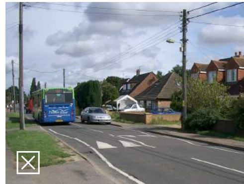
Speed bumps as a traffic calming measure for new roads should be avoided.
