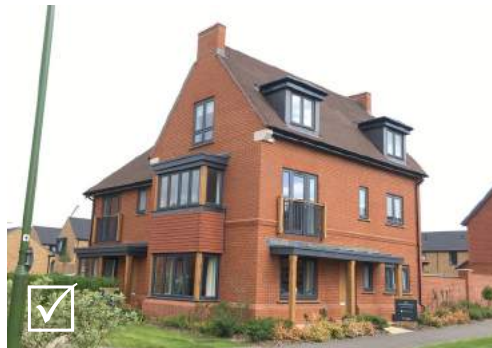
These houses address the corner well by organising the windows (and other features) so they formally address both return facades
