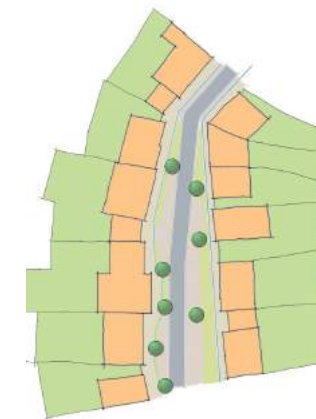
Minimize space given over to carriageway. Use the resulting space for hard or soft landscaping with parking as appropriate
