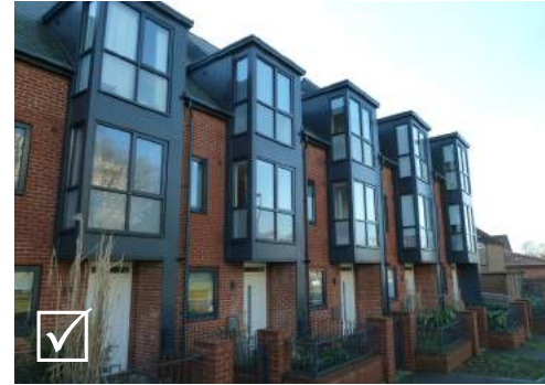
Dormers should be an integral part of the design and in proportion with the facade as in these town houses on Station Road, Burgess Hill
