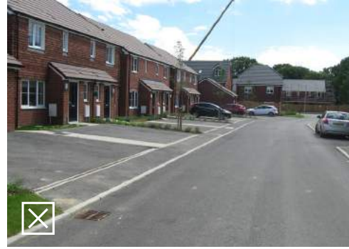
Front threshold parking reduces street enclosure and when combined with an absence of planting results in a bleak streetscape
